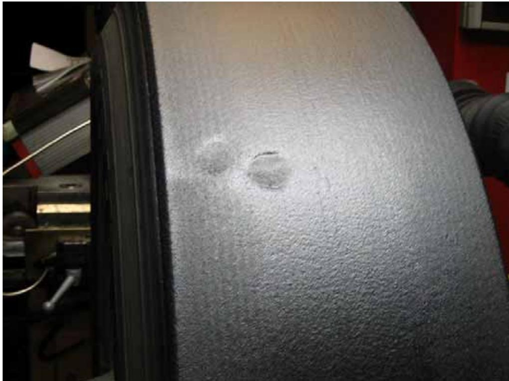
**Figure 2.10 – A Buffed Casing After Required Repair**
