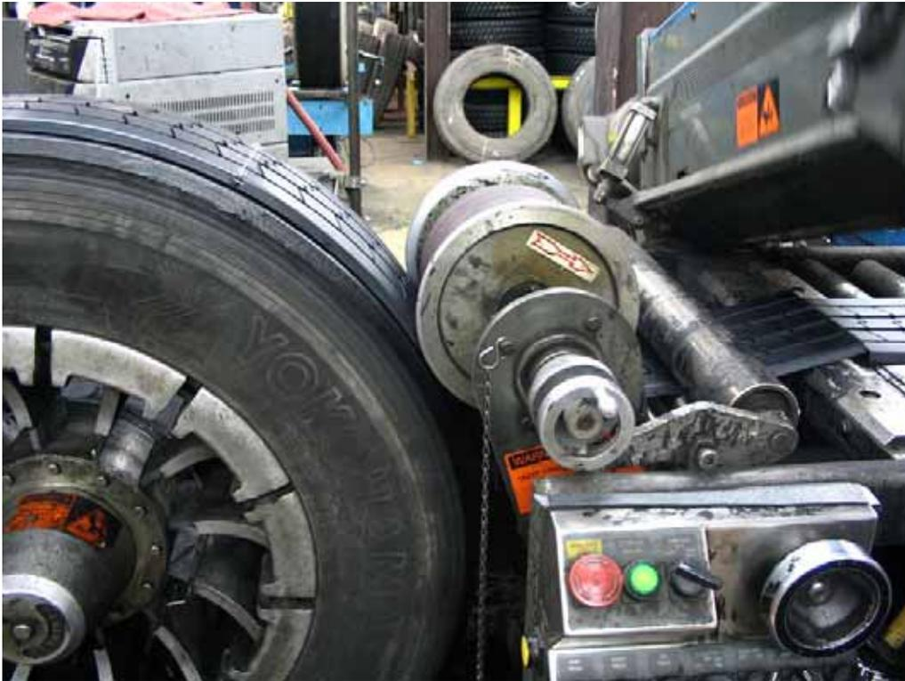
**Figure 2.11 – Application of New Tread (Precure Process)**
