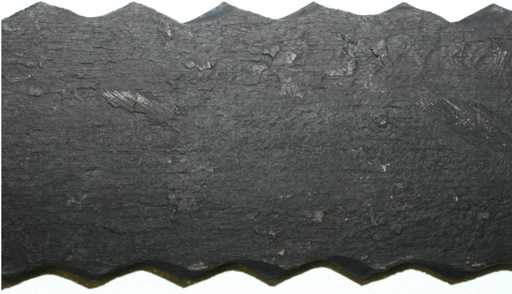
**Figure 9.18 - Manufacturing/Process Issues #4 - Bond failure at buff line**
