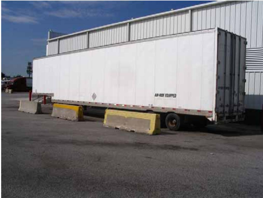
**Figure 8.8 - A 53-foot drop-frame trailer positioned at TravelCenters of America Truck Stop Lake Station, IN**
