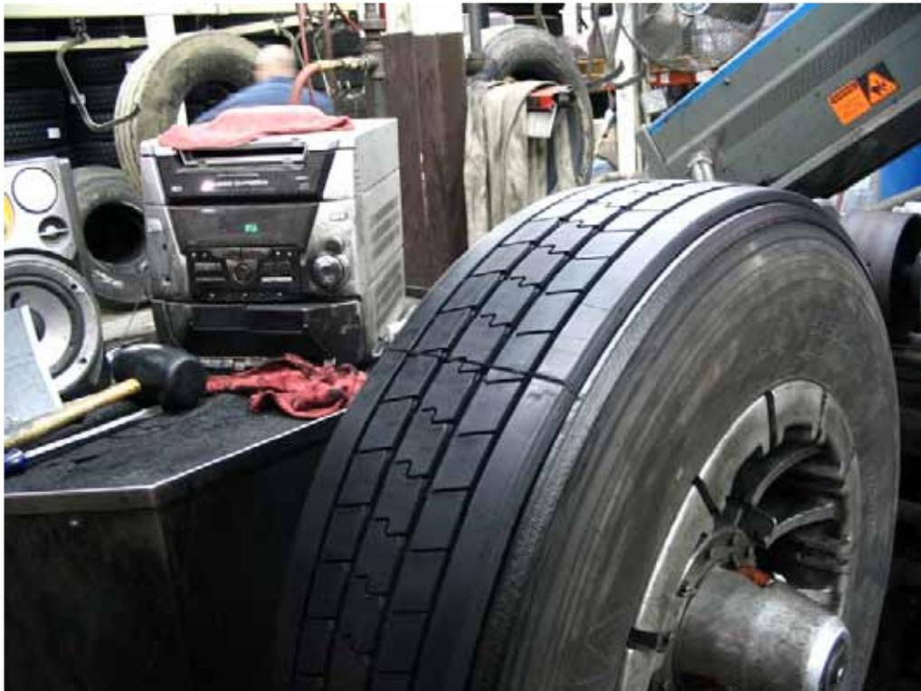
**Figure 2.21 – Precured Rubber Tread Wrapped Around Casing (Precure Process)**
