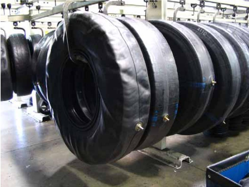
**Figure 2.13 – Pre-Cured Retread Casings Enveloped**
