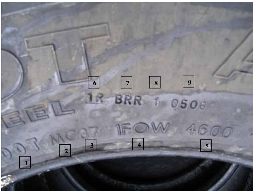
**Figure 2.27 – Tire Identification Marks on a Casing**
