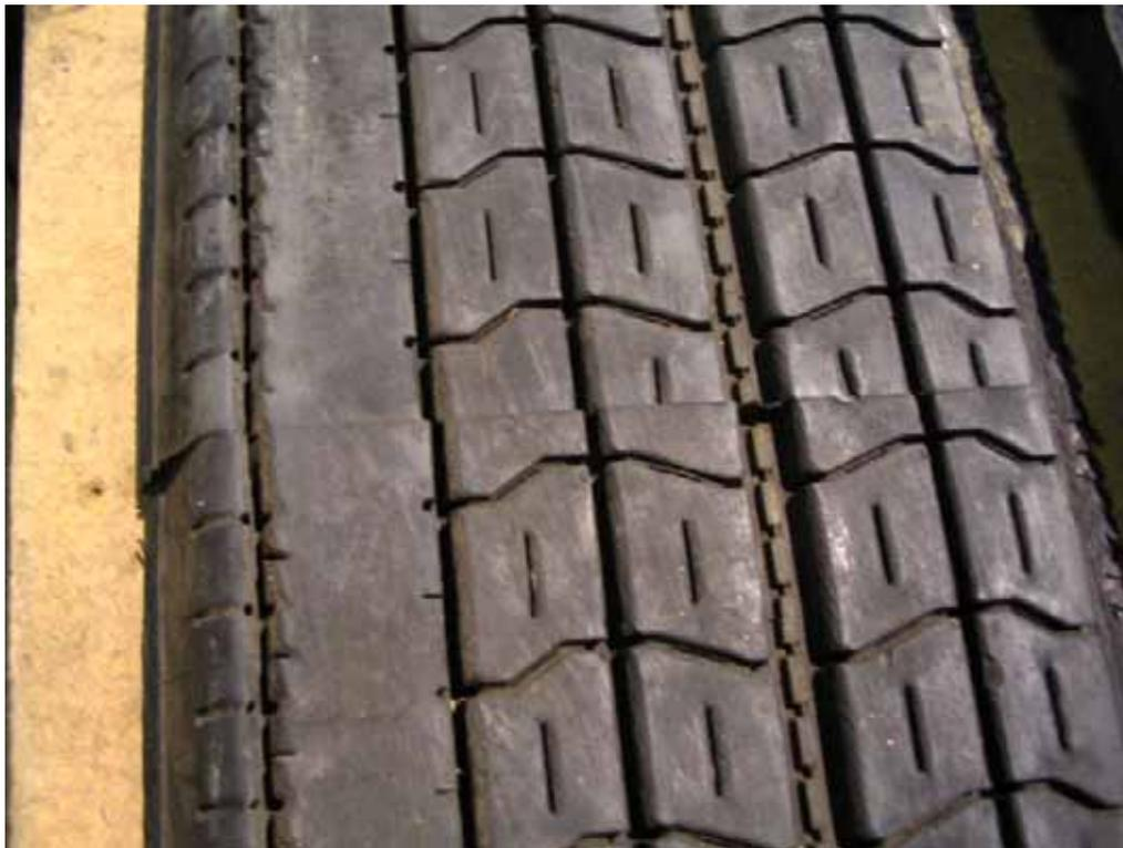
**Figure 5.4 – Misaligned Splice on a Pre-Cure Retread Casing**
