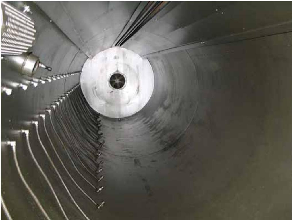
**Figure 2.14 – Inside Vulcanization Chamber**
