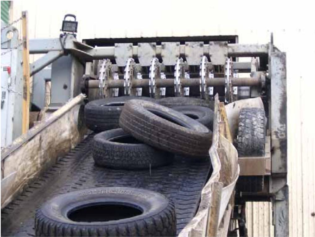
**Figure 8.14 - Rimless casings in the process of shredding**
