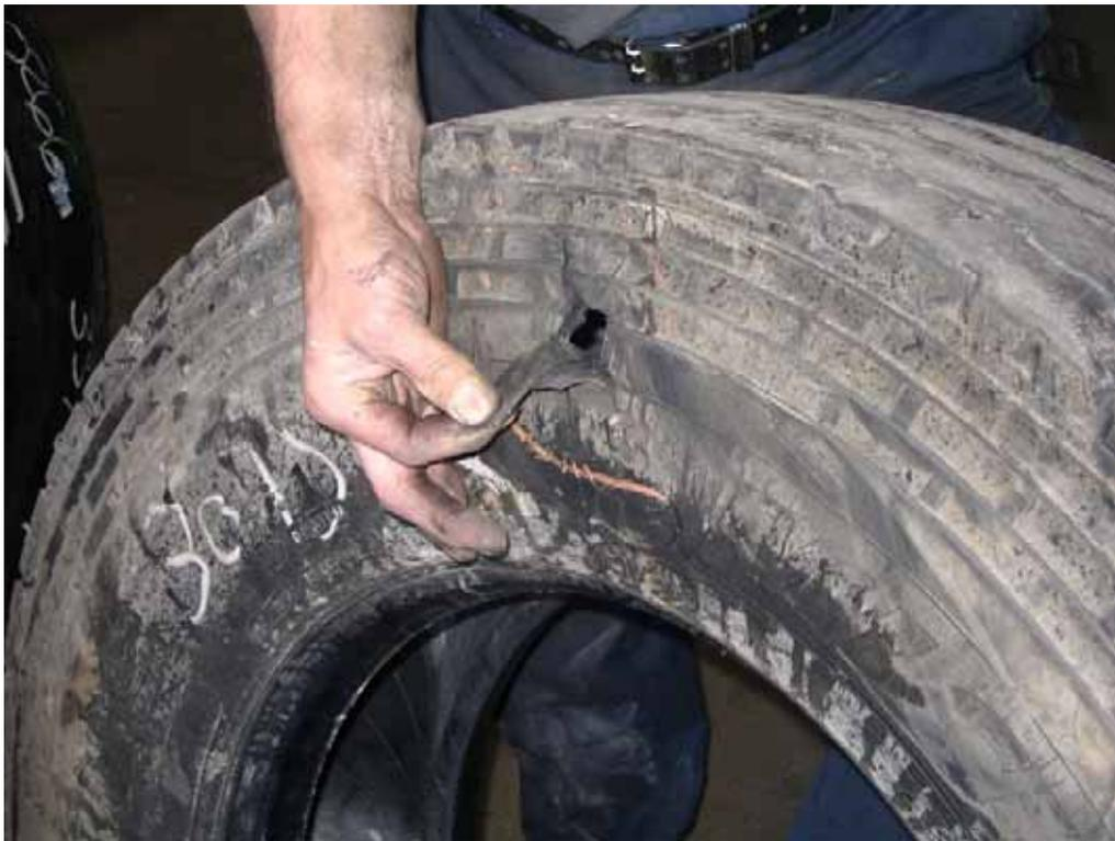
**Figure 2.5 – Hands-On Inspection of Casing**
