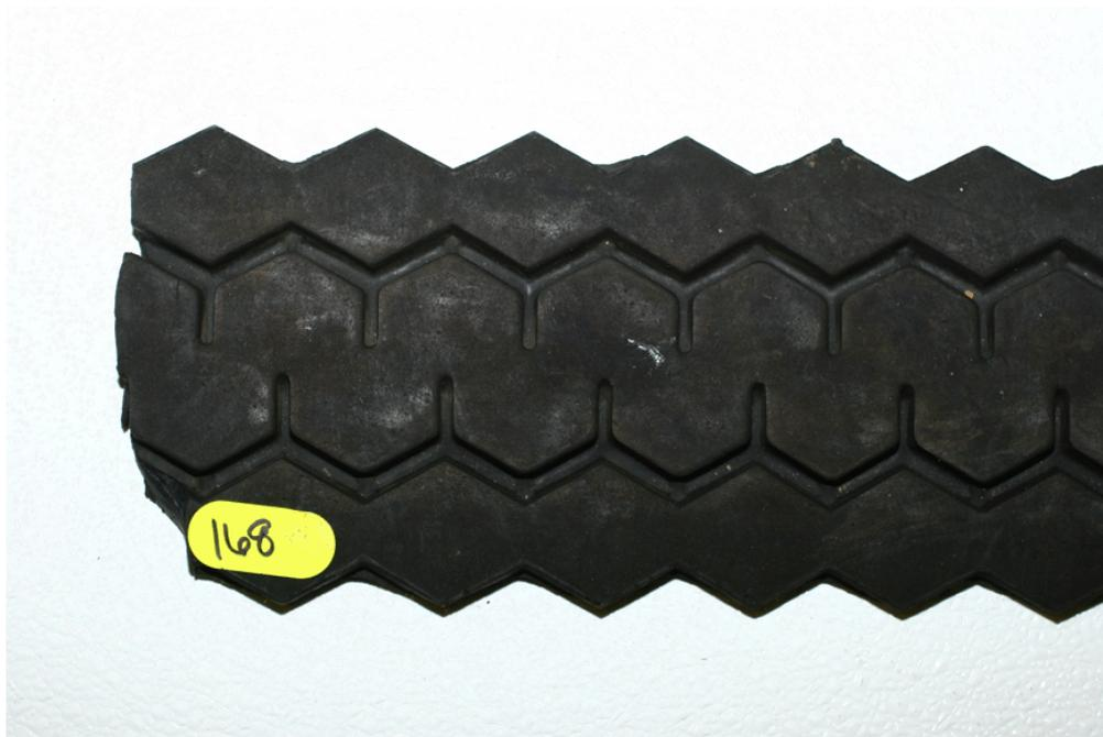
**Figure 9.17 - Manufacturing/Process Issues #3** - Bond failure at buff line
