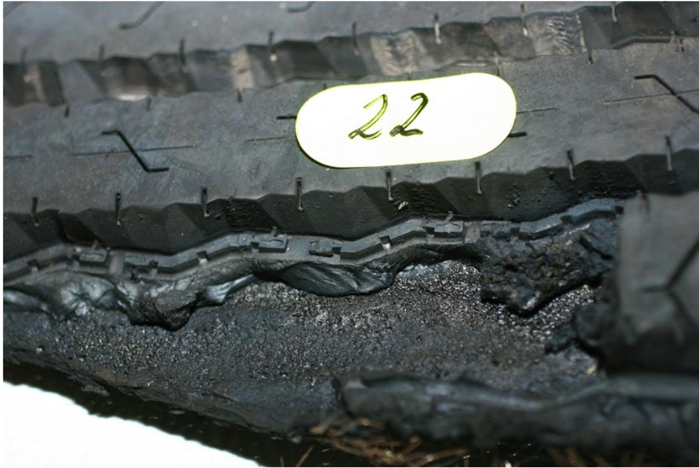
**Figure 9.6: Excessive Heat #3**
