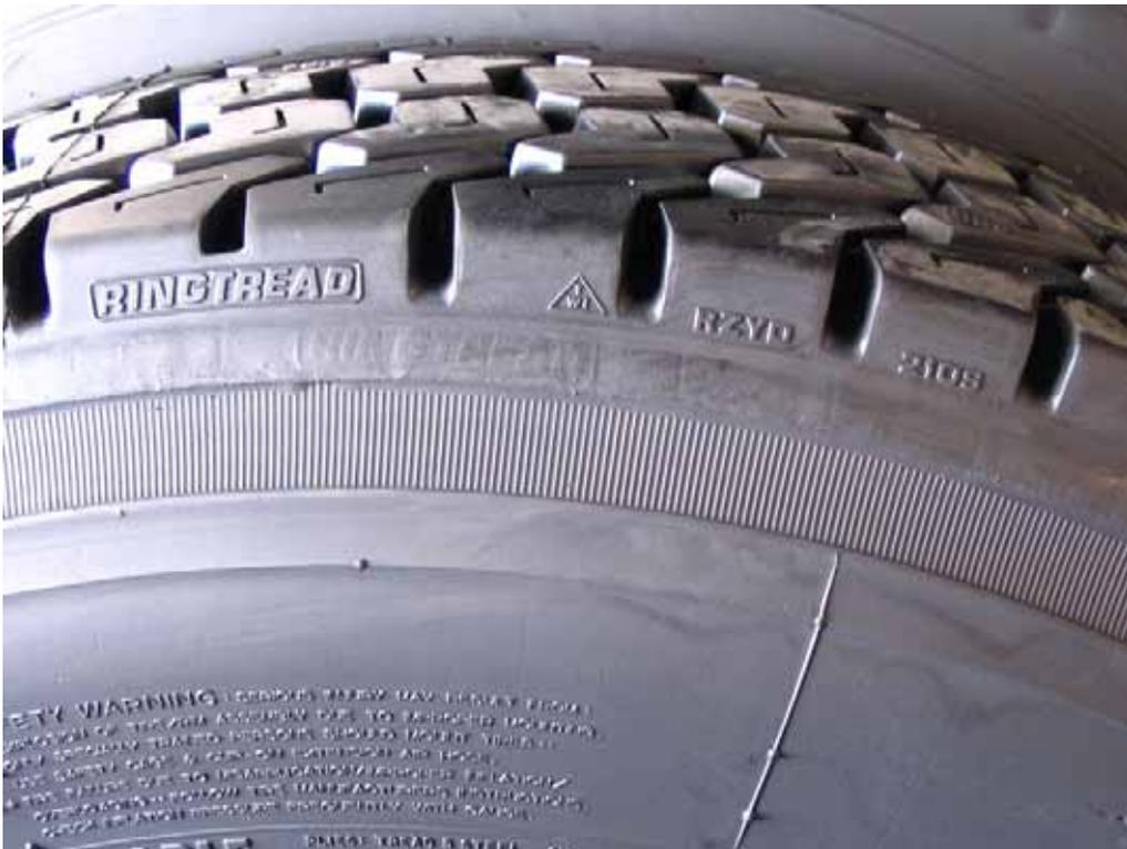
**Figure 2.16 – New Retread Casings With Ringtread Identification Markings**
