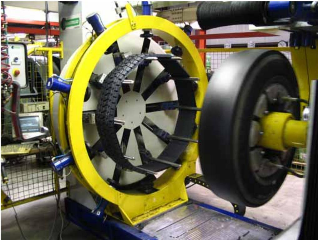
**Figure 2.12 – Application of New Tread (Ringtread Process)**
