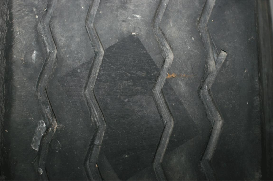
**Figure 2.25 – Tread Pattern on a Regrooved Tire**
