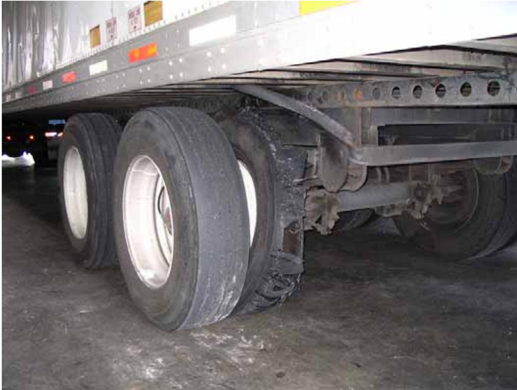
**Figure 5.1 – A Failed Medium-Duty Truck Tire**
