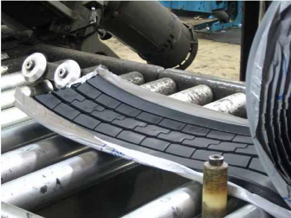
**Figure 2.20 – Precured Rubber Tread (Precure Process)**
