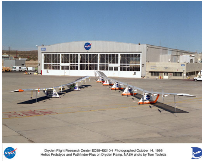
Figure 1.2: Pathfinder-Plus and Helios as samples of highly flexible Flying-Wings (photo courtesy of NASA Dryden Flight Research Center)
