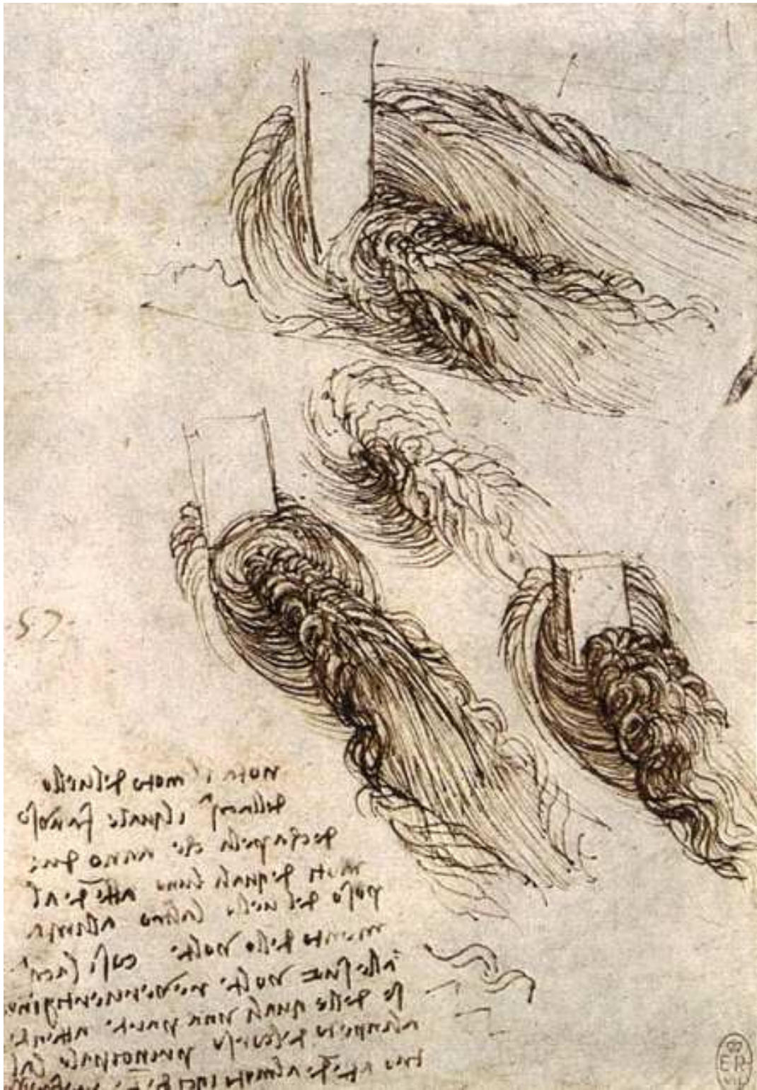
Figure 1.6: Sketch by Leonardo da Vinci in 1513 showing the wake behind a piling in a river.
