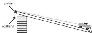
Figure 3. The washer method for measuring the force of gravity on a cart
