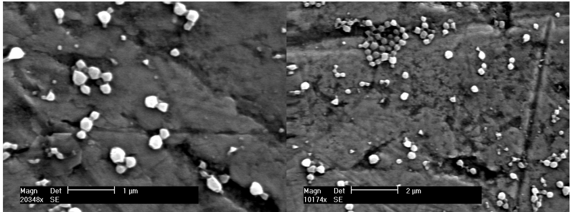
Figure 3. 8. SEM images of KTpCIPB-loaded O/W nanoparticles at different magnifications (Philips XL30 FEG SEM).
