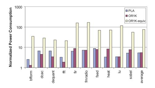
Figure 6.11: Power consumption of PLA and OR-1200 relative to single-function LA.
