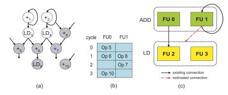
**Figure 4.4:** Wire estimation example: (a) DFG, (b) partial schedule, (c) connection diagram
