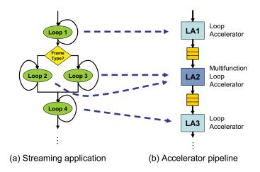
Figure 3.1: Streaming application mapped to pipeline of loop accelerators.
