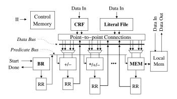
Figure 6.8: Template for programmable loop accelerator.
