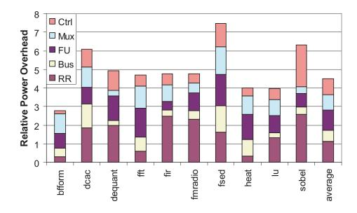
Figure 6.13: Power consumption breakdown of PLA generalizations.
