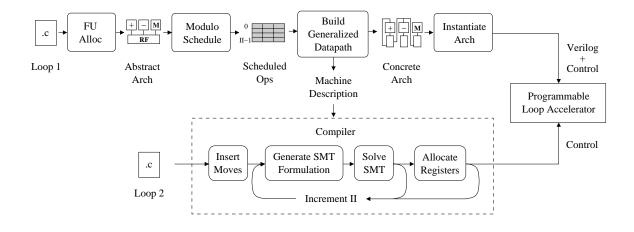
Figure 6.9: Design and compilation flow for programmable loop accelerator.
