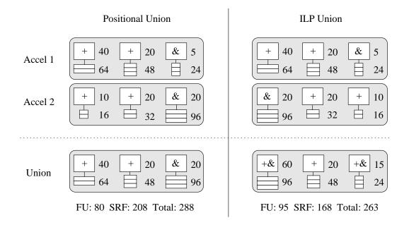
**Figure 5.2:** Example of union techniques. Two single-function accelerators, each with three FUs, are combined using positional (left) and ILP (right) methods. The cost of each FU and SRF is shown on its right.
