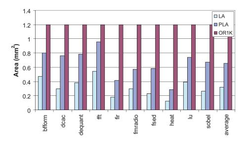
Figure 6.12: Area of loop accelerators and OR-1200.
