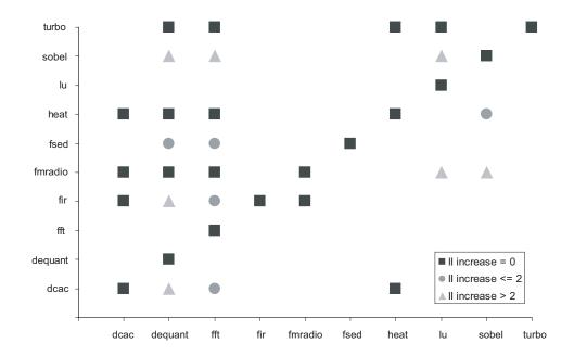
Figure 6.17: Cross compilation results. PLAs are designed for loops along the x-axis at II values listed in Table 6.1. Loops along the y-axis are then mapped onto them.
