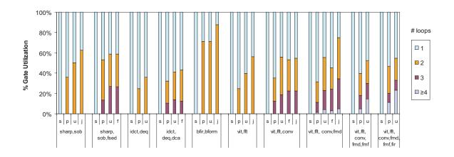
Figure 5.4: Degree of sharing of multifunction accelerator gates across loops. equivalent in cost to the full union. Thus, pairwise union is an effective and tractable method of combining accelerators.
