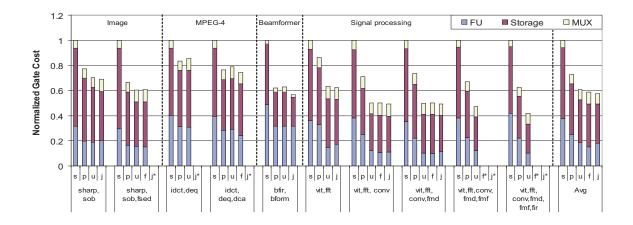
**Figure 5.3:** Gate cost of multifunction accelerators designed using sum (s), positional union (p), pairwise union (u), full union (f) (not shown for 2-loop combinations), and joint scheduling (j). \* indicates the synthesis did not complete due to problem complexity.
