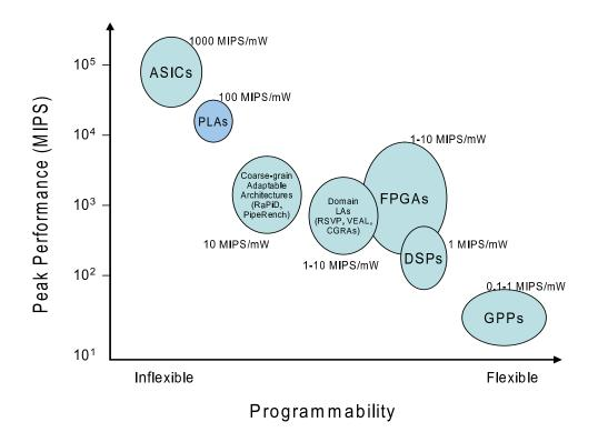
Figure 6.1: Peak performance and power efficiency of different architecture styles.
