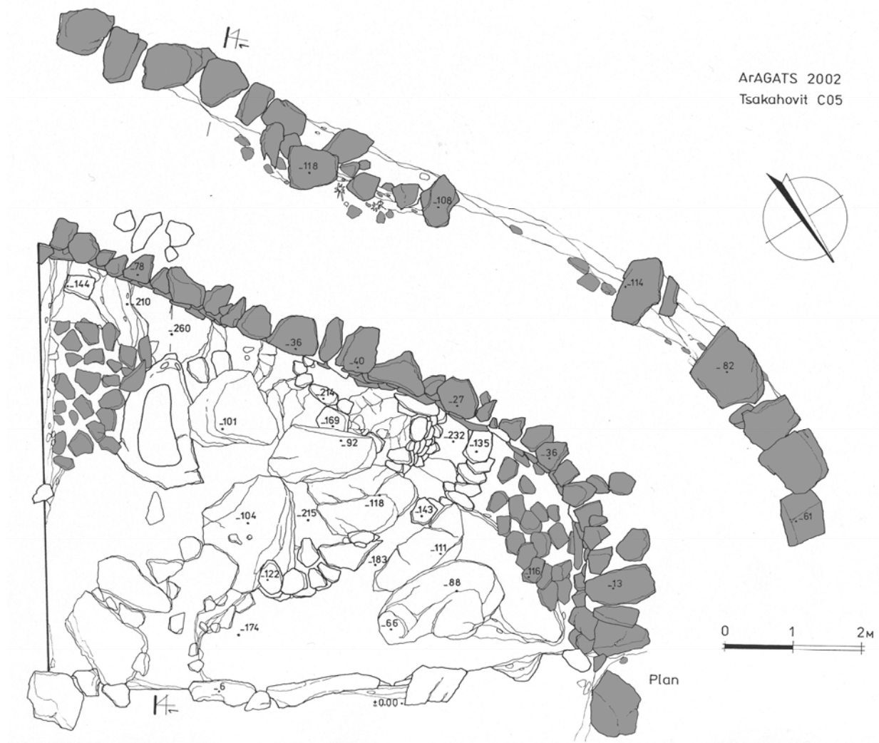
Figure 5.34 Architectural drawing of citadel operation C5. Gray areas denote Iron 3 features. (Drawing by H. Sargsyan)
