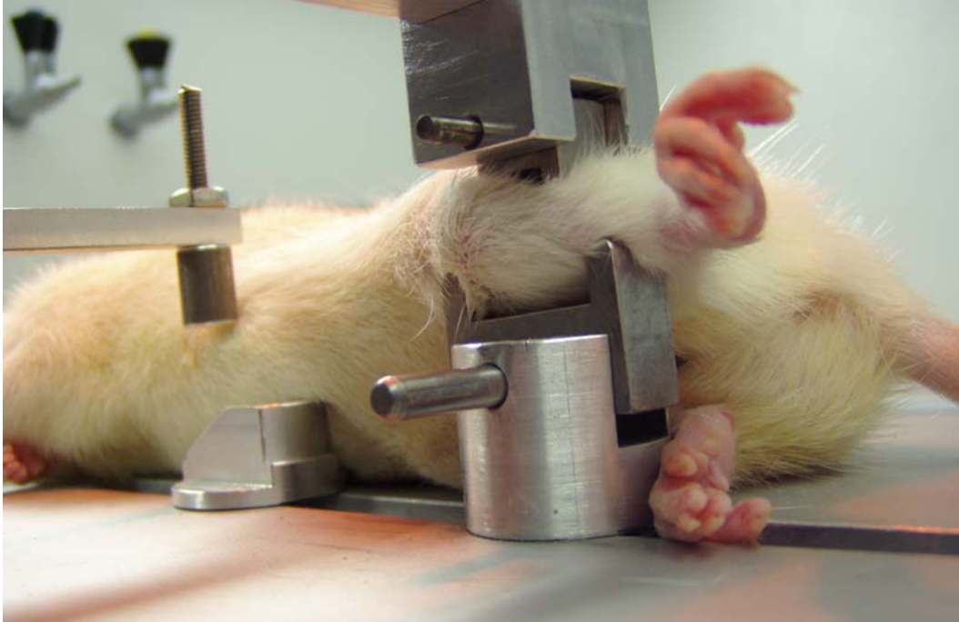
Figure 3.8. In-vivo loading of Sprague-Dawley rat
