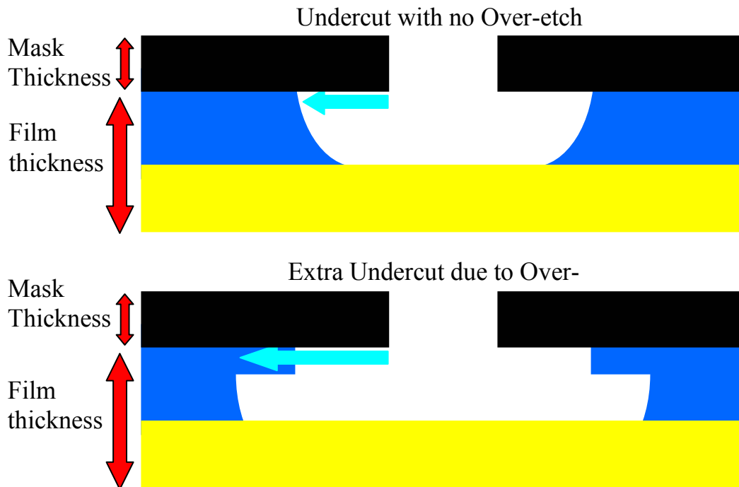
Figure 2-14: Schematic of extra undercut caused by excess over-etch.
