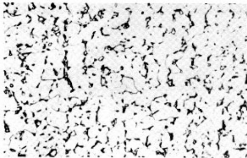
(a) Equiaxed \alpha and a small amount of intergranular \beta .
