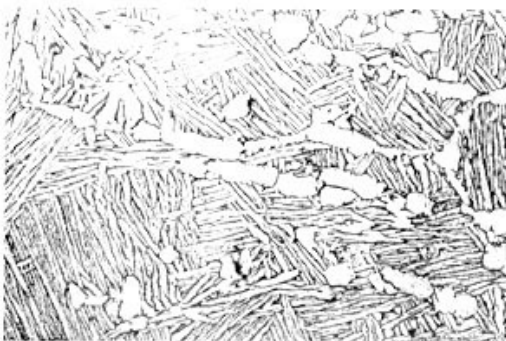
(c) Equiaxed \alpha in an acicular \alpha (transformed \beta ) matrix.
