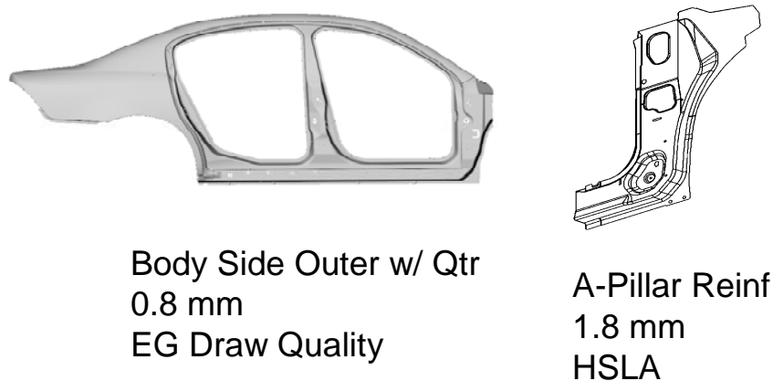
Figure 1. Stamped Parts Used for Estimating Die Tryout Performance
