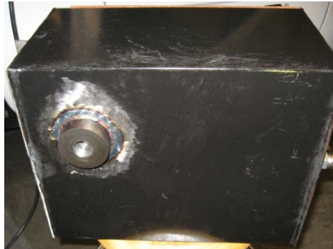
Figure 15: New Low-Side Reservoir Outlet
