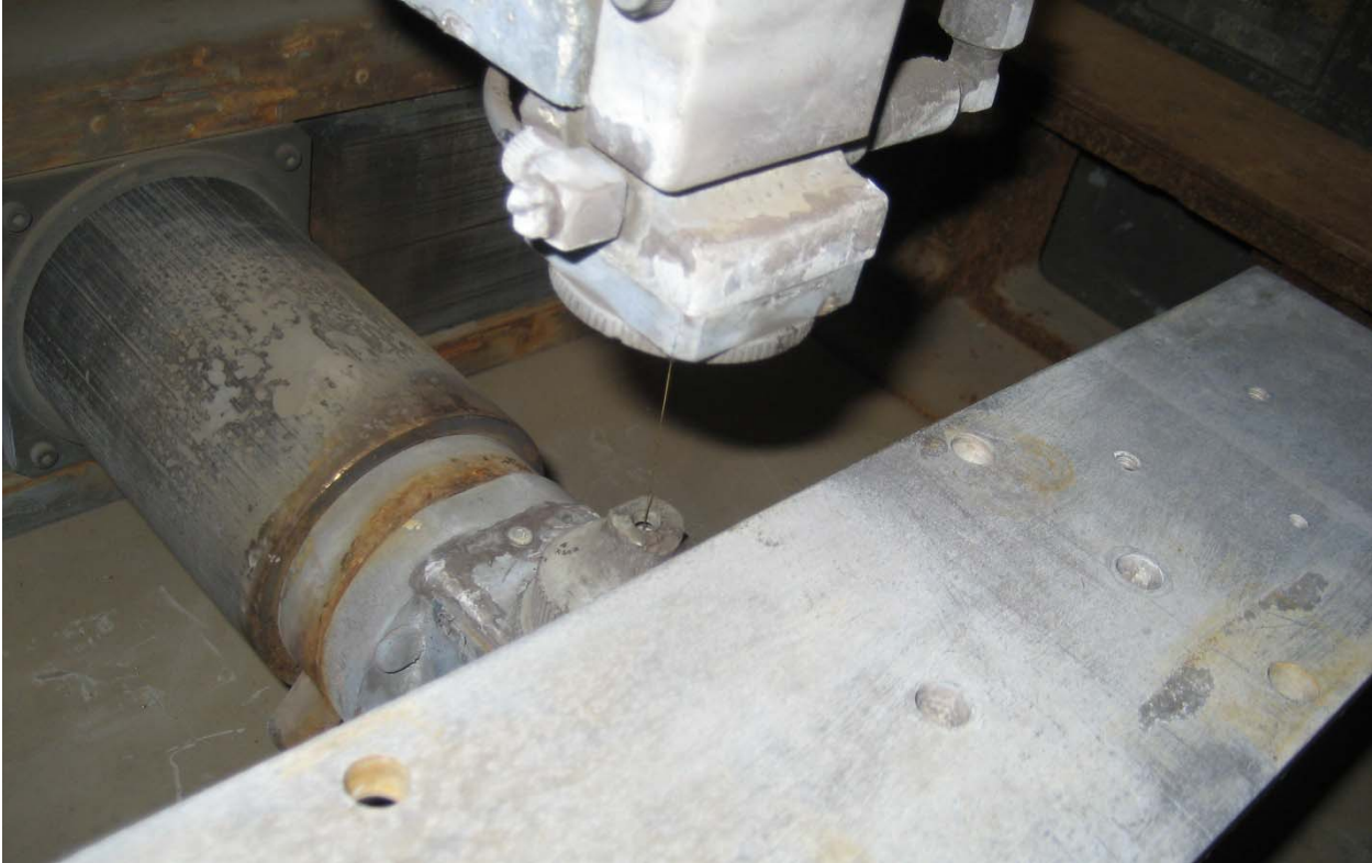
APPENDIX N.21: Electric Discharge Machine (EDM) used to manufacture gripper appendages
