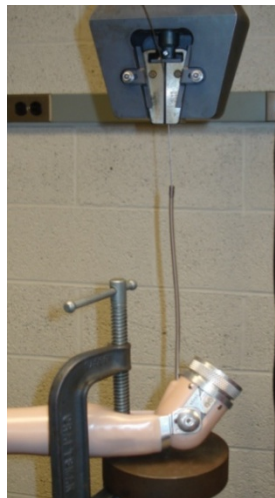
Figure 1: Elbow in Instron strain machine
