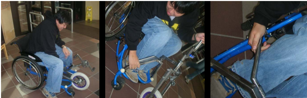
Figure A.67: The random user needed their legs to support the device (a) and had issues with the attachment arms (b & c)
