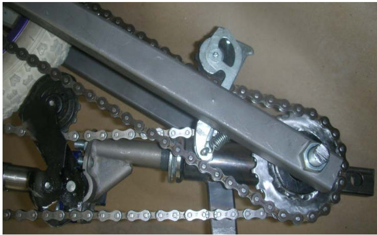
FIGURE 3 TWO SPROCKET HUB ALLOWS THE CHAINS TO STAY IN TENSION WHEN FOLDED
