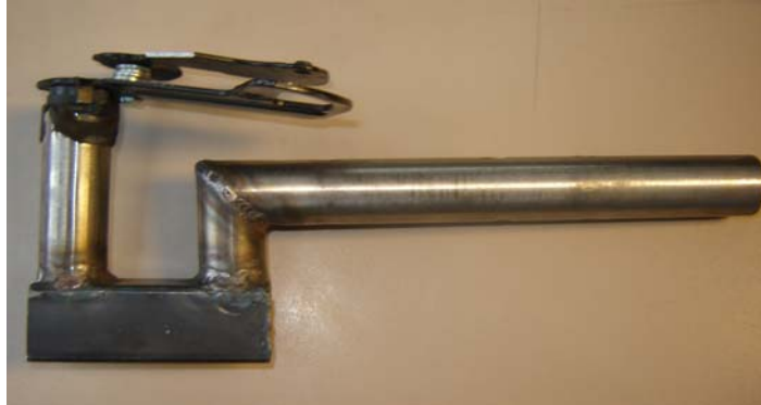
Figure C.25. Bent connection piece between steering column insert and hand crank hub
