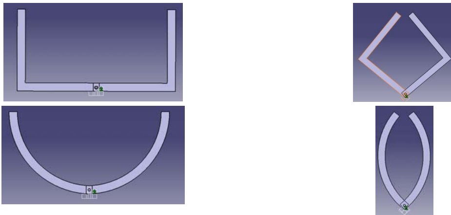
Figure A.28: Squared and rounded tubes that pivot about the same axis and have the same end points will have different widths when folded
