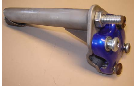
Figure C.14. Steering column shaft interior showing the handlebar bracket and angled shaft
