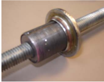
Figure C.23. Threaded axle with threaded assembly on as well as a restraining bearing collar on
