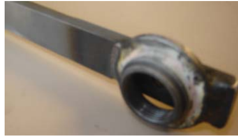
Figure C.10. Close up of reverse threaded bearing collar welded onto hand crank
