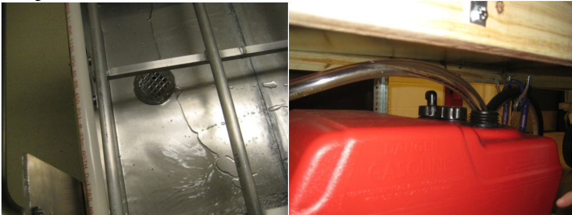
Figure 62a-b: Fluid going into the drain, through the tubing and into the container
