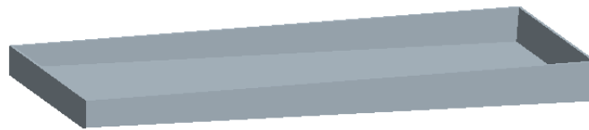
Figure 20: Fluid tray is sloped to allow fluid to flow into drain
