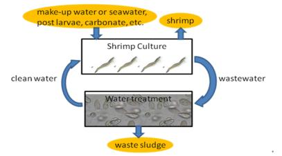
Figure 1 Schematic of a recirculating aquaculture system consisting of shrimp culture system and water treatment system.
