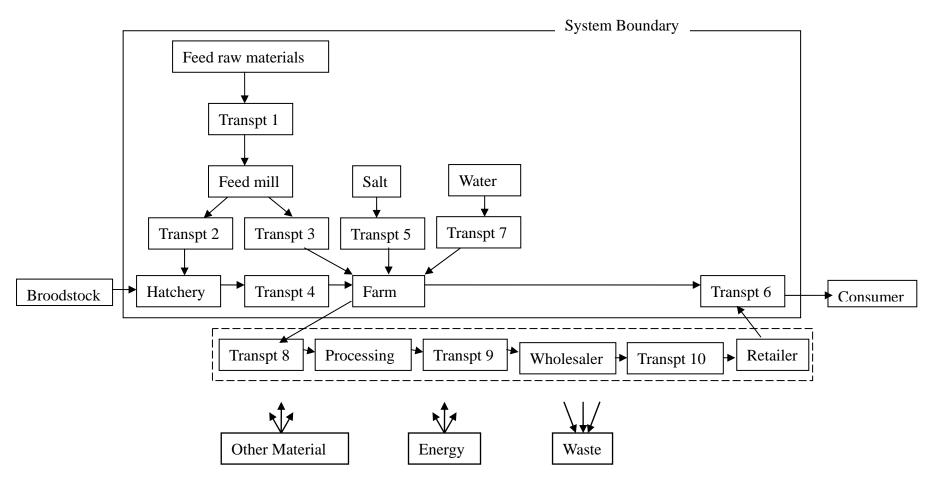
Figure 4 Detailed life cycle of recirculating shrimp aquaculture system, which highlights the scope of this thesis (excludes brood stock production and consumer stages).
