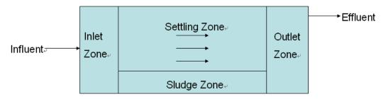
Figure 6 A schematic of four principal zones of a rectangular continuous flow sedimentation basin
