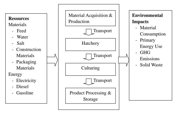
Figure 3 A life cycle schematic of the recirculating shrimp aquaculture system, analyzed in this thesis.
