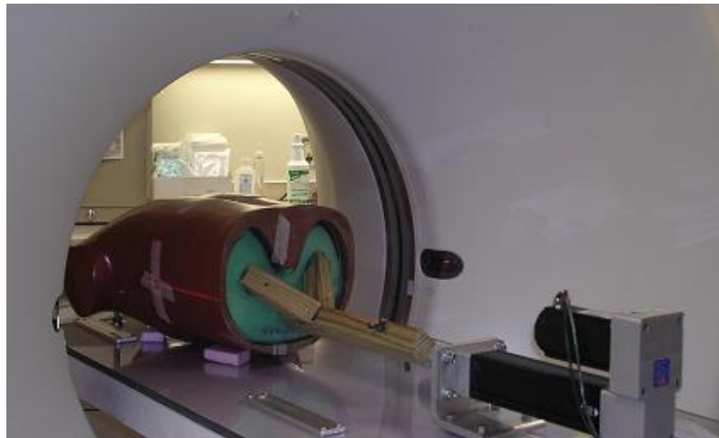
Figure III.2: The set up of the phantom and motion actuator on the CT scanner
