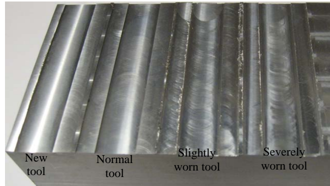
Figure 3.10: Milled slots with different tools
