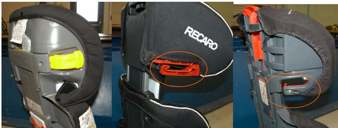
Figure 22. Difference in shoulder belt guide structures in the Compass, Recaro, and TurboBooster (left to right). The Compass (left) retained the belt most successfully in this test series.
