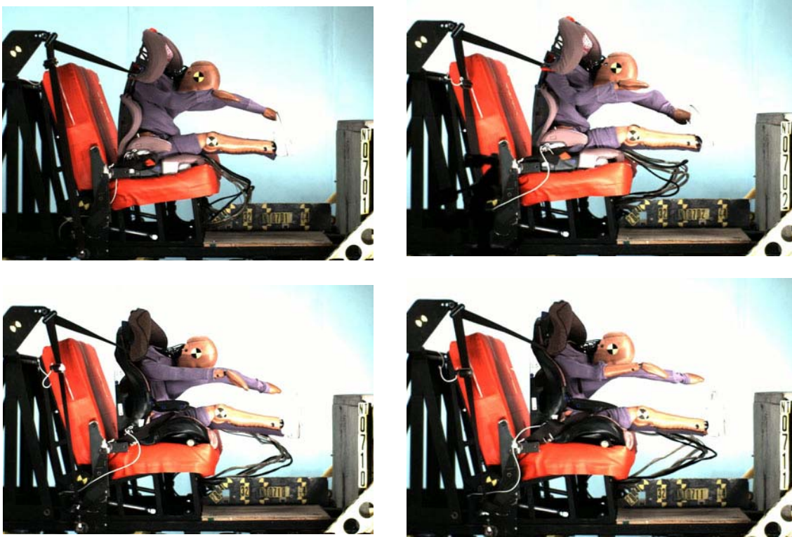
Figure 4. Comparison of peak excursions. Top row: booster A, bottom row, booster B. Left: ~60 N lap belt tension, right: ~8 N lap belt tension.
