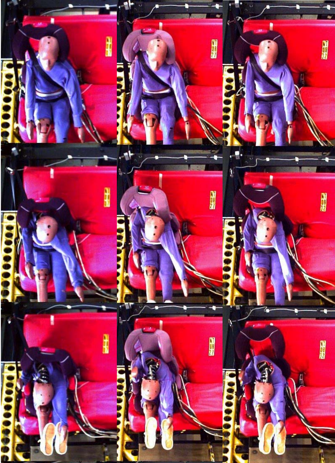
Figure 25. Kinematics of TurboBooster (left), TB with modified slot (middle), and rigid TB. Frames from top to bottom are from times 80, 100, and 120 ms.
