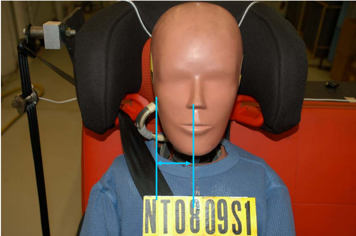
Figure 1. Illustration of shoulder belt score (SBS) measurement.
