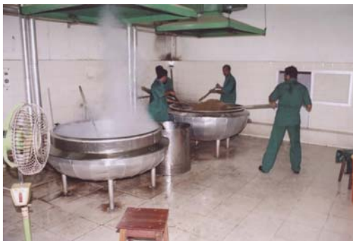
(Photo 6-4: Industrial pharmaceutical workers prepare an Ayurveda-based asthma medicine in a steam- heated aluminum cauldron that is in the shape of a traditional brass vessel)
