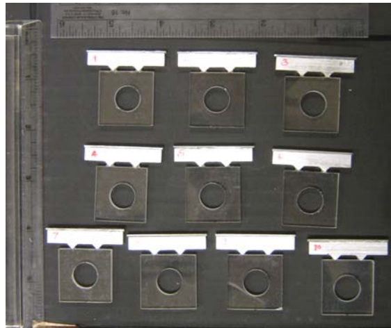
Figure 4-6 Glass plate sensors and schematic test setup for the calibration
