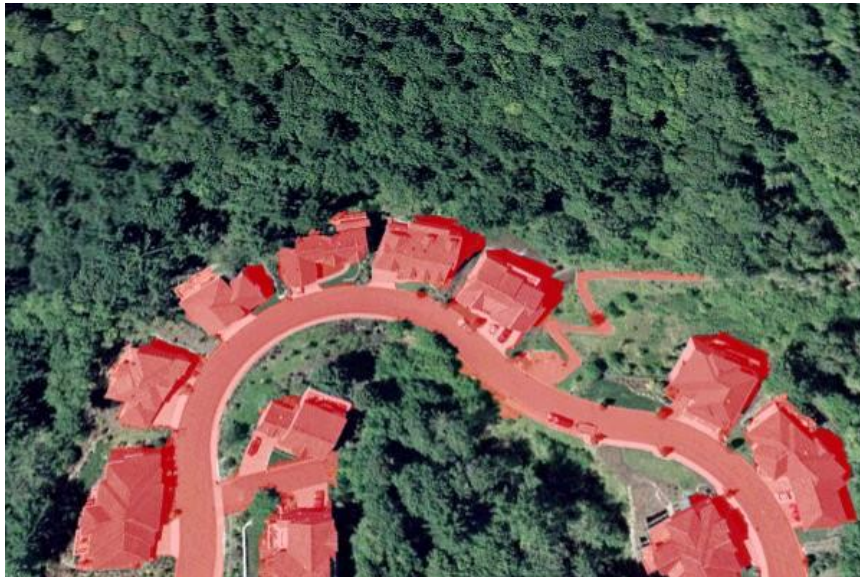
Figure 2.2 Measuring percentage of impervious surface
