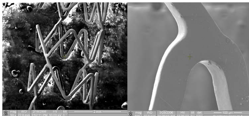
Figure 6.3: Micrographs obtained using SEM showing the morphology of the polymethacrylate/Cu(II)-cyclen on CVD coatings on the stainless steel stents after expansion. No defects in the coating were observed even after mechanical expansion of the stent.
