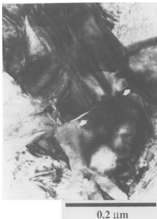
Fig. 19. TEM micrograph of 3Y-TZP after fatigue shows a lenticular microcrack along the grain boundary (as indicated by arrows).
