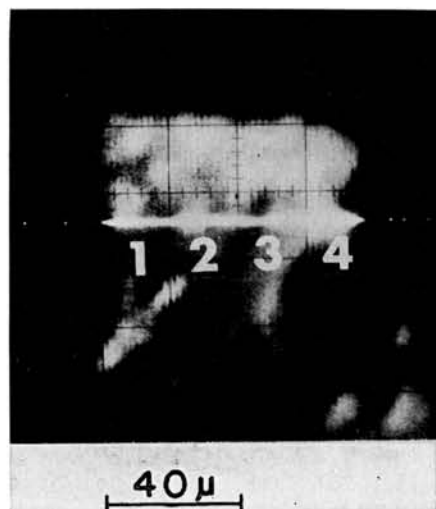
FIG. 7.—Back-scatter pattern of same area shown in Figure 2. Line designates path of electron beam during scans for the elements.
