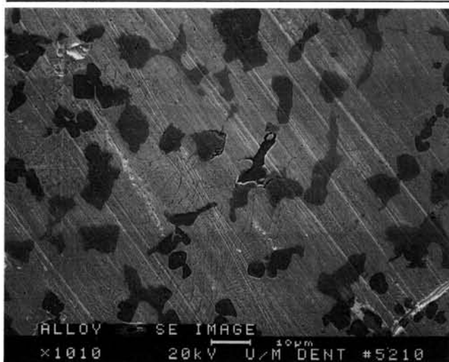
Fig. 1—Scanning electron micrograph (SEM) of alloy 8 containing 51.5 Au, 28.1 Ni, 12.6 Ga, 3.9 In, and 3.8 Pd (at. %). The dispersed phase contained Ni and Ga, the matrix phase consisted of Au and In, and Pd was segregated.
