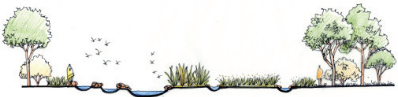
Figure 6.11: Section along the constructed wetland on the site which goes across the forebay, high marsh area, the low marsh area and the surrounding forests
