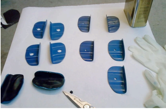
Figure 33 shows ArchFlux plates being coated in polyurethane
