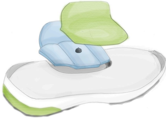
Figure 28 shows an exploded view of the shoe sole, ArchFlux frame, and ArchFlux bladder
