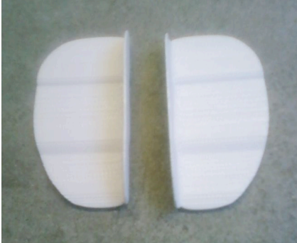
Figure 32 shows printed ABS plate models
