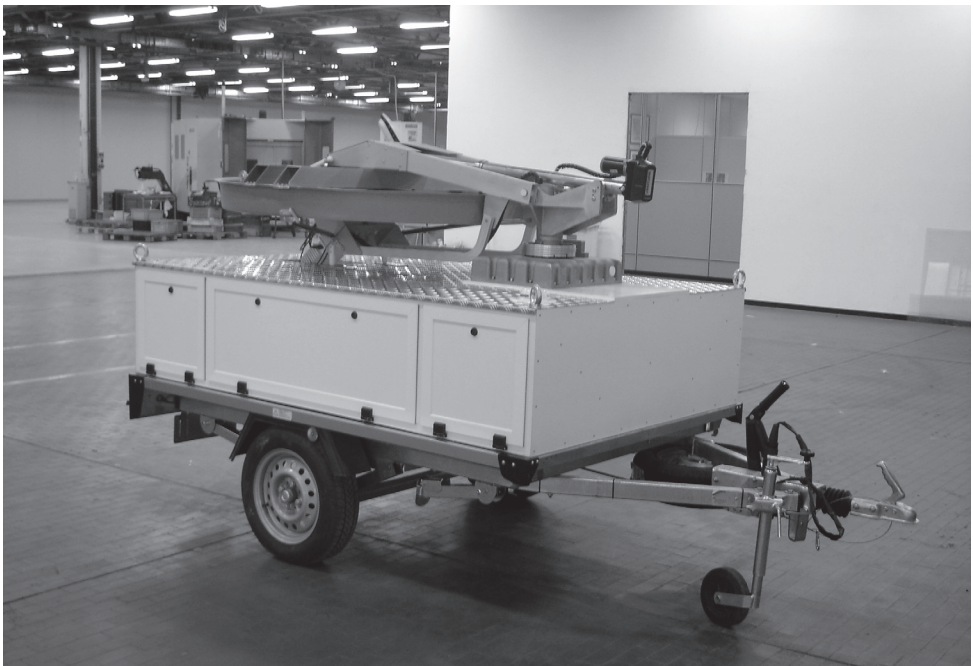
Figure 2 The MOBSAT Access Point providing Wireless LAN IP connectivity to a GEO satellite
