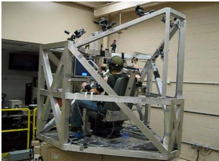
Figure 5.1: Reach Experiment on the Ride Motion Simulator
