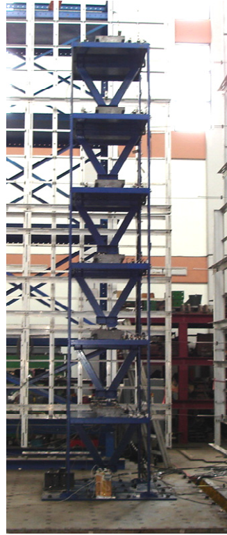
Figure 5.11. Six-story laboratory steel test specimen.
