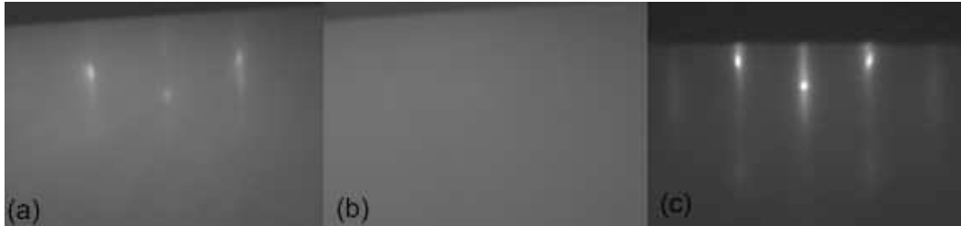
Figure 3.18: RHEED patterns (a) upon growth of 0.5ML SrO at 50°C (b) upon growth of 2ML SrTiO 3 at 50°C (c) upon recrystallizing SrTiO 3 at 600°C
