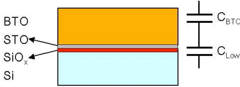
Figure 3.25: Schematic showing lowered apparent dielectric constant due to an interfacial SiO x layer
