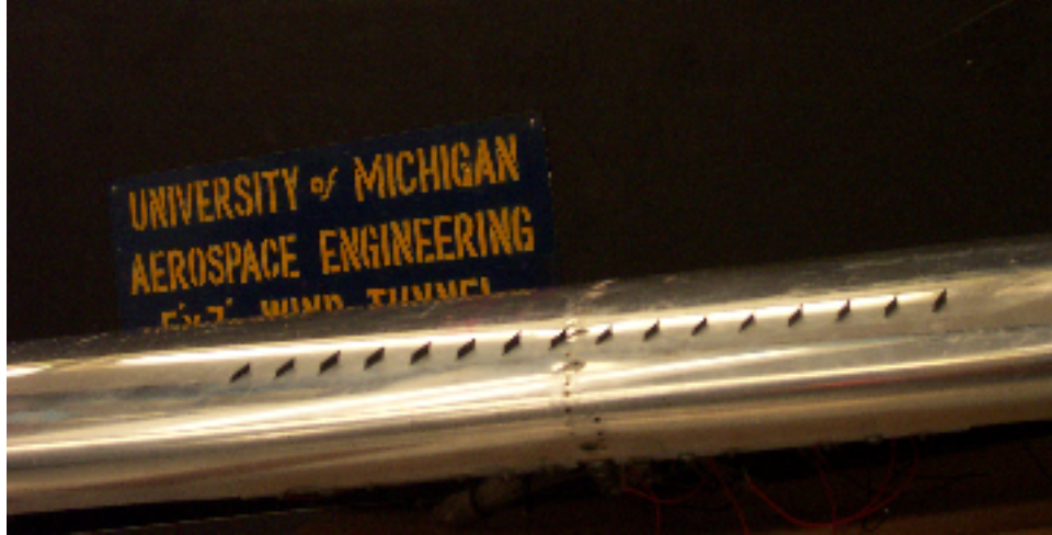
Figure 5: Vortex generator array installed in the pitching wing model.
