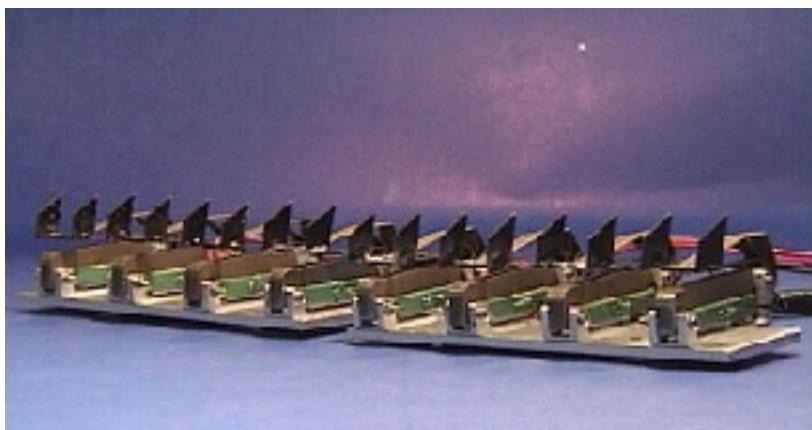
Figure 7: Eight actuator-amplifier array with 16 vortex generator blades.
