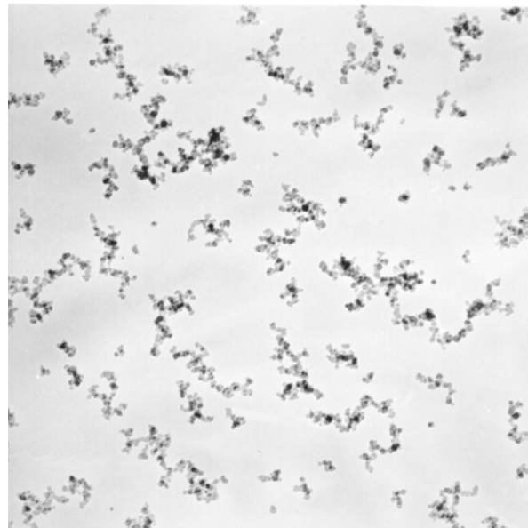
Fig. 1 TEM photograph of soot aggregates along the axis and near the start of the soot formation region of an acetylene-fueled laminar jet diffusion flame burning in an air coflow at 1.0 atm.
