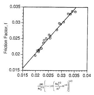
Figure 1: Turbulent Friction Correlation for Hydromagnetic Channel Flow
