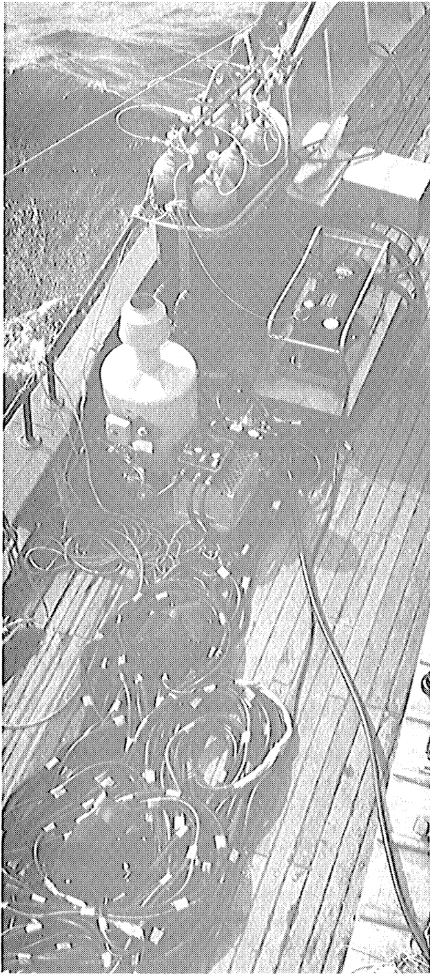
FIGURE 5-2. Air supply systems. (a) Bank of 240 ft 3 high pressure air cylinders, high pressure air compressor, hot water heater, and umbilical on deck of R/V Inland Seas (Photo by R. Anderson). (b) Compact low pressure air compressor and separate air receiving tank. (c) High capacity diesel engine driven low pressure compressor, 72 ft 3 /min, 250 lbs/in 2 , size: 48 x 64 x 44 inches, weight: 1080 lbs. (Photos from Bolstad Engineering and Manufacturing)
