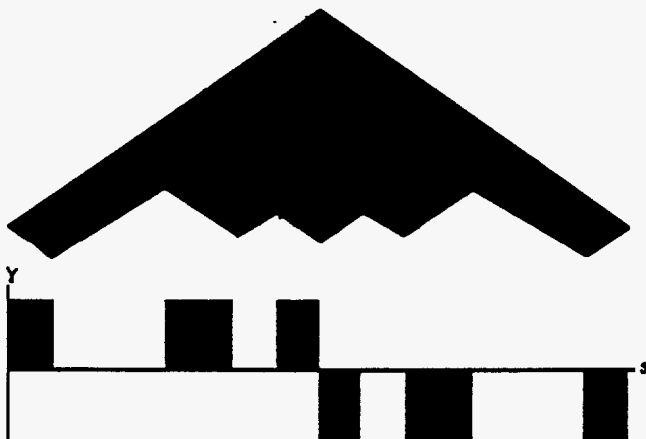
Figure 3 B-2 planform and circulation density distribution
