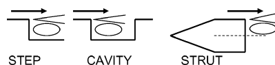
Fig. 2 Schematic showing that step, cavity, and strut flameholders consist of the same components: a shear layer located between the freestream and the recirculation zone.
