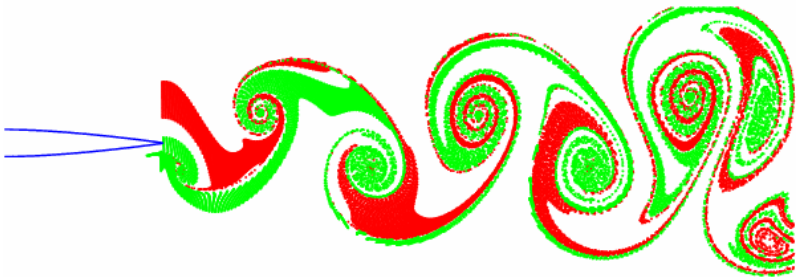
Figure 12. Streakline plot of flow over plunging airfoil NACA0012 at Re = 20,000 and reduced frequency of 3.93.
