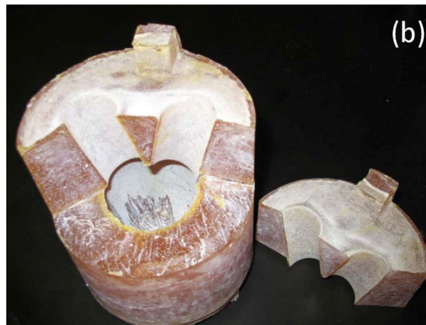
Figure 4.3 Negative molds for the inner (a) and outer (b) surfaces made of Hyperflex.
