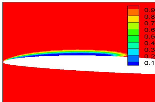
(b) NACA66MODE hydrofoil \mu_T/\mu_L|_{inlet} = 10^3 , effective Re=2000
