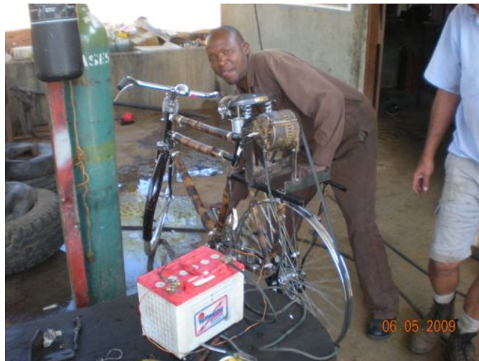
Figure 5.5: Final product charging a battery
