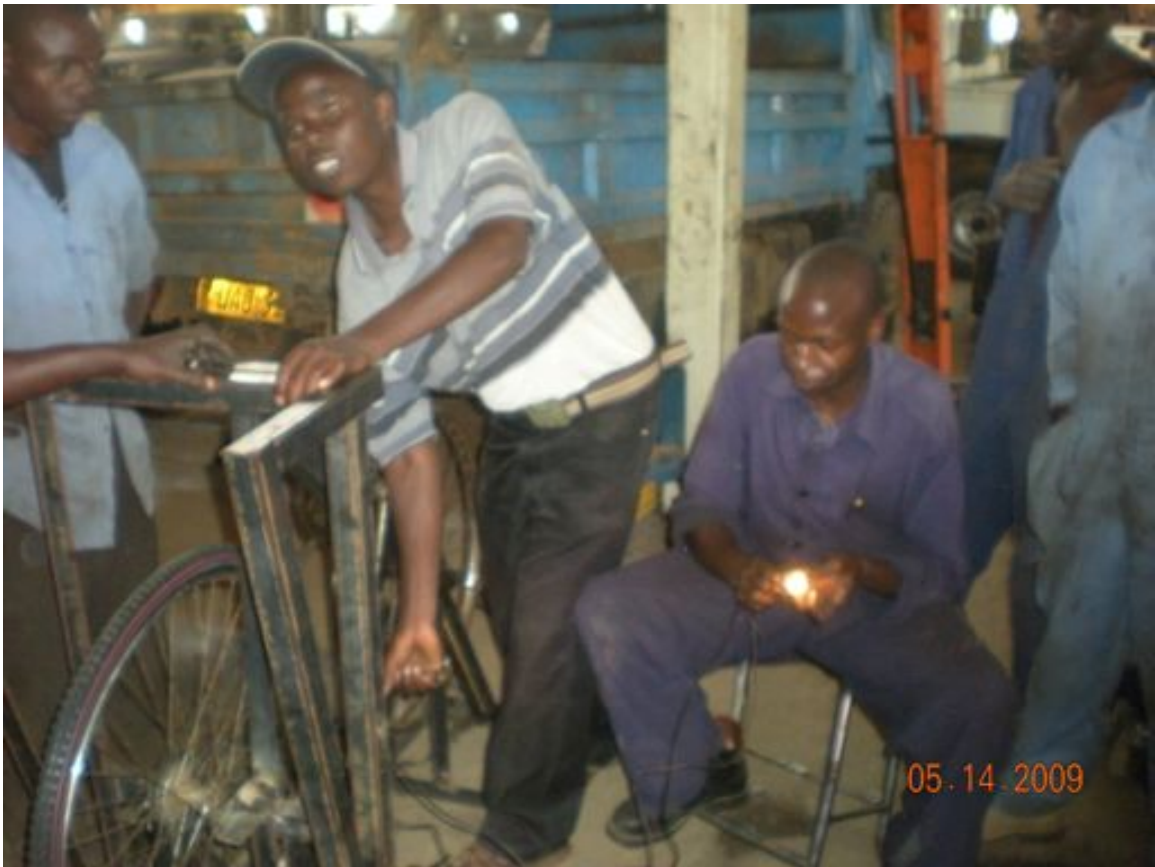
Figure E.1: Bicycle generator lighting up a bulb. Built by the local technicians at St. Joseph's Technical School
