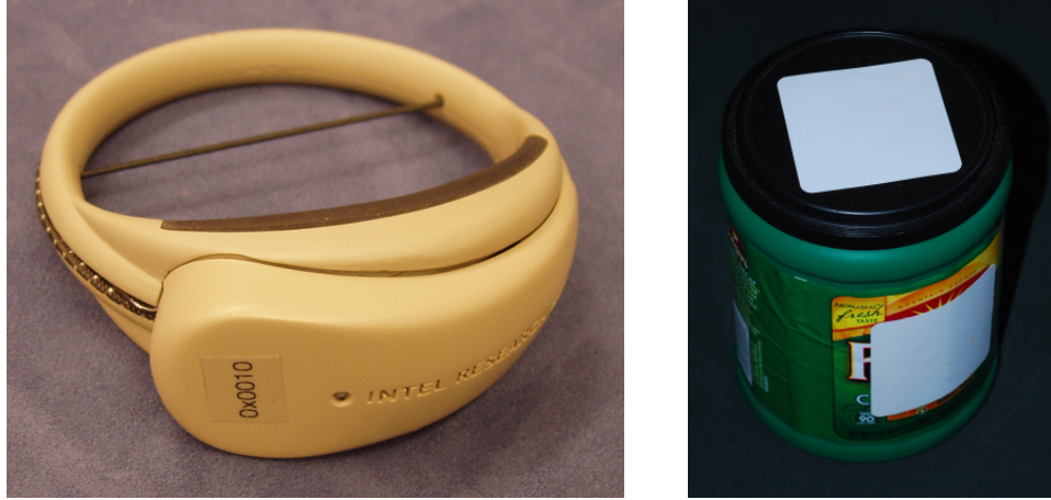
Figure 3.1: RFID Equipment Used in the Experiment. The Intel iBracelet RFID Reader (l) and Canister of Ground Coffee (r).
