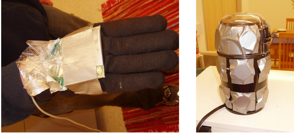
Figure 2.1: Equipment Used in the Study. The Glove with an RFID Reader Attached (l) and the Coffee Grinder with Several RFID Tags Attached (r).
