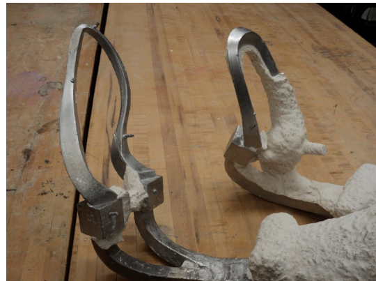
Figure 22: Aluminium castings with gas releases still attached.
