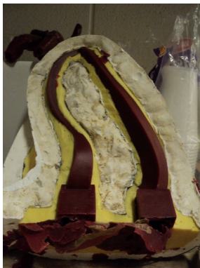
Figure 21: Wax in rubber mold prepared for lost wax process.
