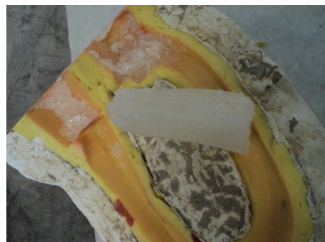
Figure 19: Sodium Acetate being taken out of mold. The brittle nature of the material prevented a clean release.
