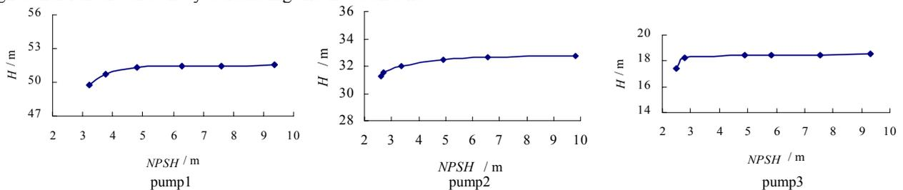
**Figure 6 Cavitation performance prediction curve on design condition**
