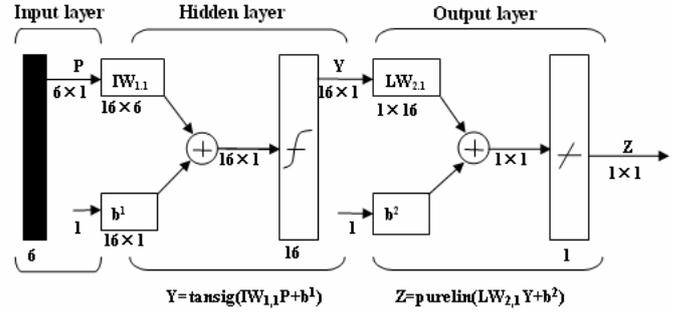
Figure 1 Architecture of BP neural network
