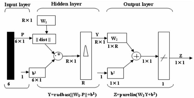
Figure 2 Architecture of RBF neural network
