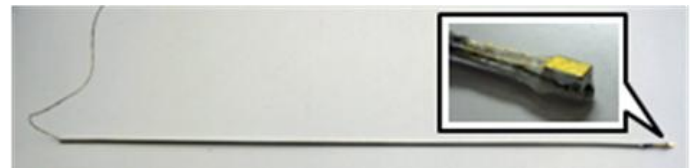
Fig. 4 Temperature probe with DT-670-SD silicon diode sensor.
