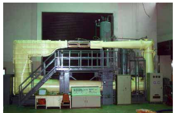
Figure 5: Cavitation tunnel at Seoul National University
