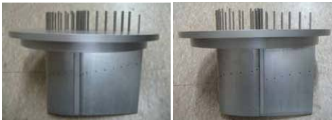
Figure 6: Models for surface pressure measurement
