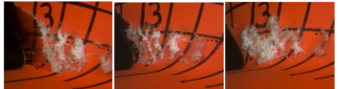
Figure 15: The potentially erosive vortex group cavitation shed downstream an upstream collapsing sheet near the root of a propeller (leading edge on the left). Experiment carried out in SSPA’s cavitation tunnel [22].
