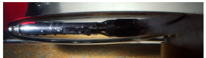
Figure 6 Mo II CoSCIS operating in the SAFL water tunnel.
